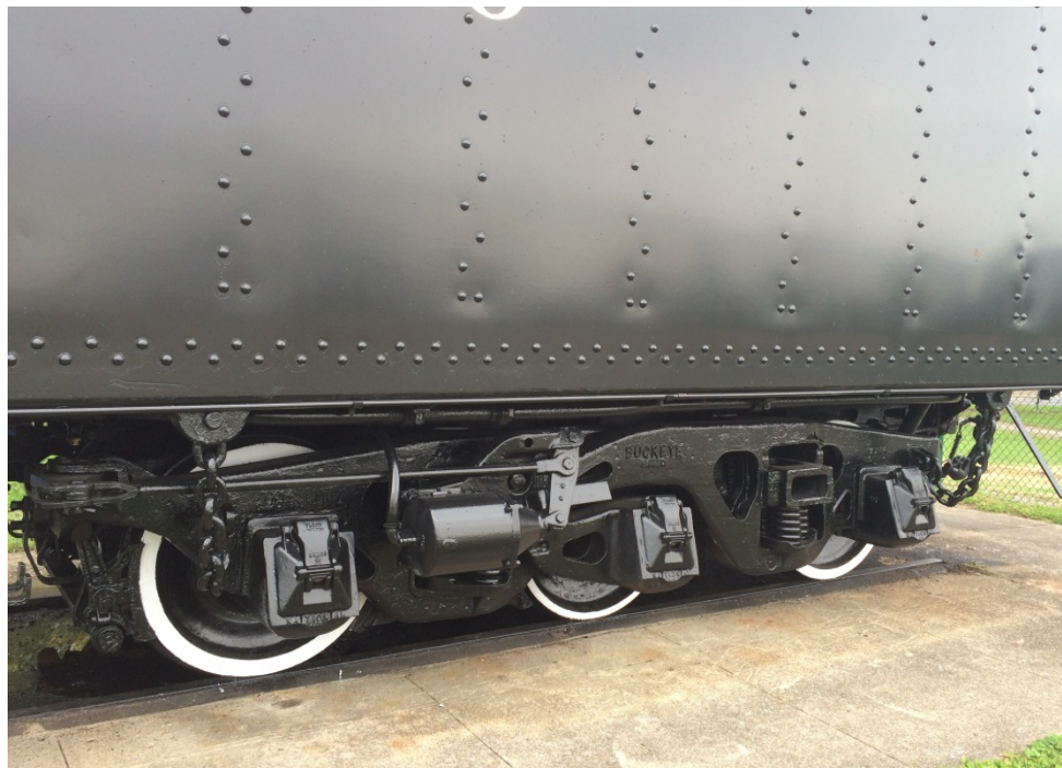
Example of Buckeye Steel Casings Locomotive Tender truck made by Buckeye Steel. Washington Court House display of C&O #2776.
